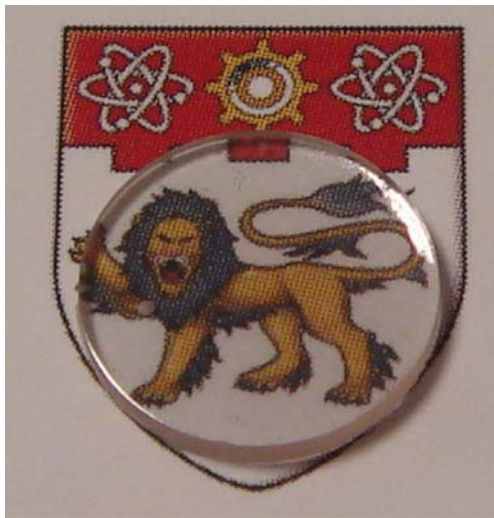
Fig. 4 Photograph of mirror-polished YAG transparent ceramics on the logo of our university
